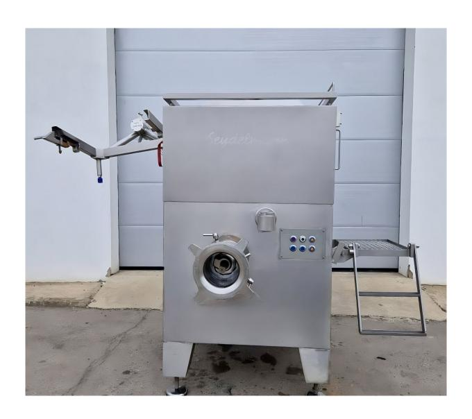
Grinder with mixer 200 mm hole plate diameter
